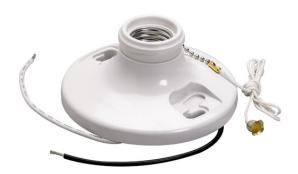
Medium base, phenolic, pullchain, 4 terminals with tri-drive screws, fits 3 1/4" to 4" boxes, with cage neck, 6" Leads. White.
