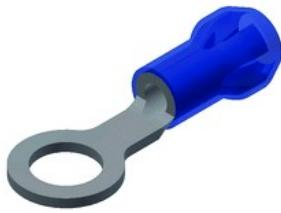
Copper Terminal, Ring Tongue w/o Inspection Hole, Wire Range 16-14 AWG, #8-#10 Stud, Nylon Insulated, Tin Plated, 600 Volts Max.
