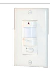
Fits decorator wall plates with only 1/2" protrusion. 120 volts. Gangable. Full 180° view covers 1000 sq. ft Works with electronic ballasts. Can be wired in parallel. LED indicator, wallplate included. Can also be used as a ceiling sensor. Must have hot and wires in box.
