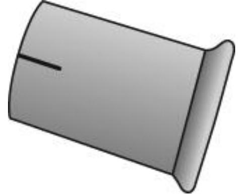
*A two-piece, internally threaded expansion anchor with four equally-spaced longitudinal slots extending from the bottom end of the outer shield, inside of which sits a pre-assembled dilating plug.*
