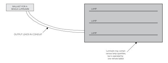
Note: Recommended output lead lengths and remote mounting distances should not be exceeded.
