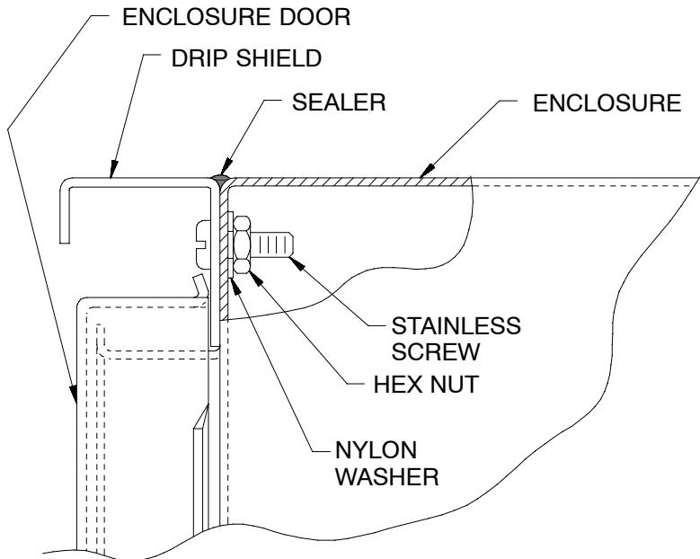
2. Use the drip shield to locate and drill one of the end holes first, using a 7/32 inch drill. Align drip shield and install a 10-32 screw through the shield and enclosure. Then drill the remaining holes using the drip shield as a guide. Install the remaining screws, nylon washers, and nuts as shown.
