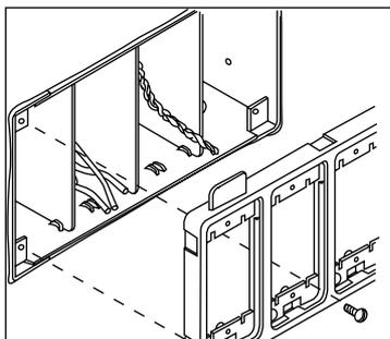
5. Install self-levelling WSC07-6 device mounting bracket.
