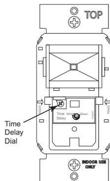
Adjustment controls are located behind the front cover of the unit and are clearly labeled.
