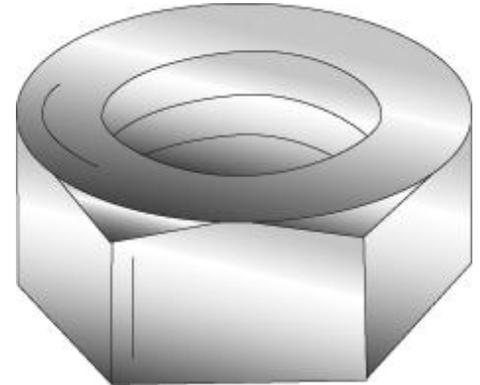
*A six-sided internally threaded fastener with flat tops and chamfered corners.*
