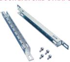
Straps mount to the door bar. Used to mount accessories to the door. Constructed of 16 gauge steel with plated finish. Holds up to 100 lb.
