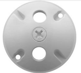
Die cast round covers with one or three 1/2" holes. Fit 4" round boxes. Supplied with thick foam rubber gasket and two #10-24 stainless steel screws. 3 hole cover comes with one die cast 1/2" close-up plug.
