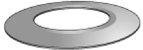
*A disc spring, or "Belleville washer", consists primarily of a convex disc supported at the outer periphery by one force and an opposing force on the center of the disc. Disc springs are used singly, or in stacks, to achieve a desired load and travel.*
