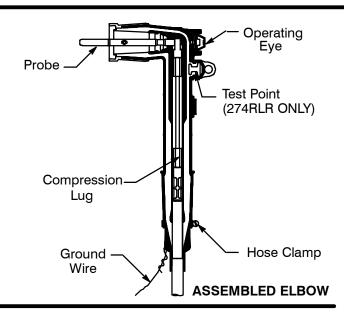
**CAUTION:** Lubricate test point cap and assemble tightly.
