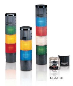
The Litestak® LSH Horn is a piezoelectric unit that employs a ceramic element which expands or bends when voltage is applied, generating a single tone. Model LSH can be used as a stand-alone audible device (with the LSB pipe/surface mount base or LSBS surface mount base) or combined with the Federal Signal Litestak light modules to create a combination audible/visual signal.
