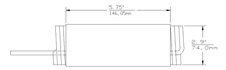
NOTE: WHEN APPLIED TO CABLE, 600ECS's LENGTH WILL INCREASE UP TO 8" DEPENDING ON CABLE O.D.
