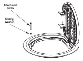
CAUTION: CRFB4 Floor Box has two sets of Cover Attachment Holes. Use the attachment holes furthest away from the mounting screw.
