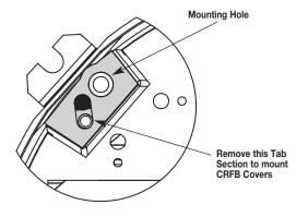
8CT and 8CTC COVERS: Open the lid and insert Cover Attachment Screws through Sealing Washers and attach Cover Flange to CRFB4 Box.
