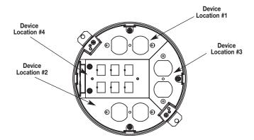
2. If necessary, use bushing(s) and wire tunnel to facilitate wire and cable routing. Remove the temporary cover and the (5) #8 hex screws securing the device mounting plate and lift it out of the box, exposing the internal barriers. Remove necessary knockouts and twistouts between compartments to allow desired wiring layout. Replace the internal barriers and reinstall the device mounting plate back in its original orientation.
