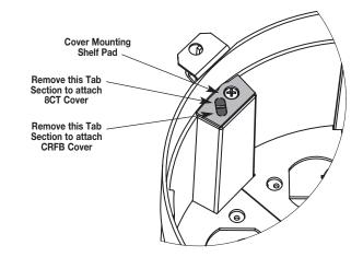
8. CRFBBTC and CRFBCTC COVERS: Open the lid and insert Cover Attachment Screws through Sealing Washers and attach Cover Flange to CRFB4 Box.
