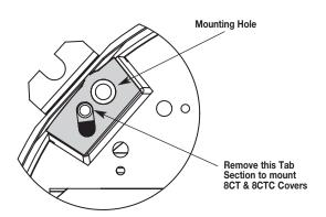
10. FOR 8CT FLUSH STYLE COVERS INSTALLED IN WOOD FLOORS: Create a pocket 9-3/8" diameter [283mm] x 7/32" [5.6mm] deep, concentric with mounting hole from step 1. Place gasket (supplied with cover) in counterbore and attach cover. Apply sealant between edge of hole and flange.
