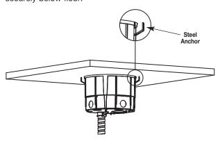
6. Install the floor covering prior to attaching the cover. For carpet installations, the temporary cover plate can be used as a template.
