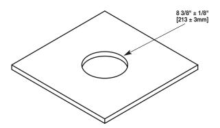
NOTE: Floor thickness range (including floor covering 3/8" – 2" [9.5mm – 51mm].
