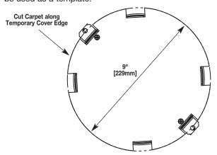
Attach cover to box. Remove the appropriate shelf pad tab, exposing the threaded attachment hole. Secure cover to box with screws provided.
