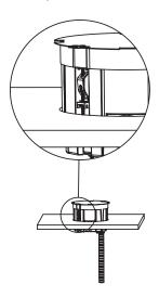
5. Tighten mounting screw until steel anchor is adjusted securely below floor.
