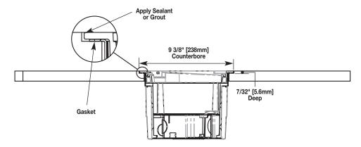
For factory wired CRFB4 access floor boxes, use Installation Instructions supplied with Walkerflex® Modular Wiring Systems.
