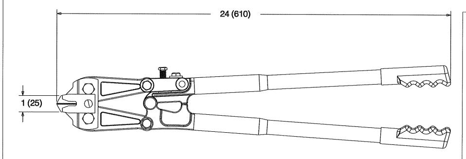
Panduit tool number WGCT-M is used to cut cable tray.
