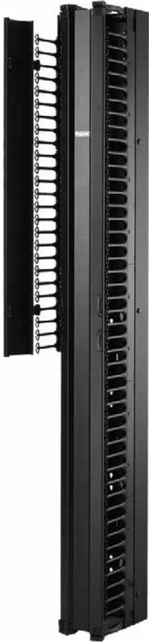
MAXRACK™ Air baffle and Vertical Cable Manager accessory kits ensure CISCO switch compliance. They provide the required cold air access and provisions for high-density cabling. Baffles and cable manager uprights made of aluminum; supporting fingers made of composite. Finish is RAL 9005 black light-textured, low-gloss polyester powder paint.
