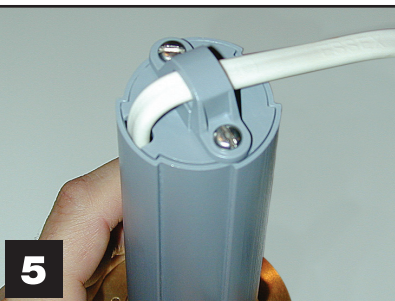
Figure 5 - Secure wire clamp on bottom of tube.
