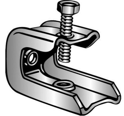
*Beam and flange clamp assemblies are used to hang conduit, cable, etc. from a buildings structural support.*
