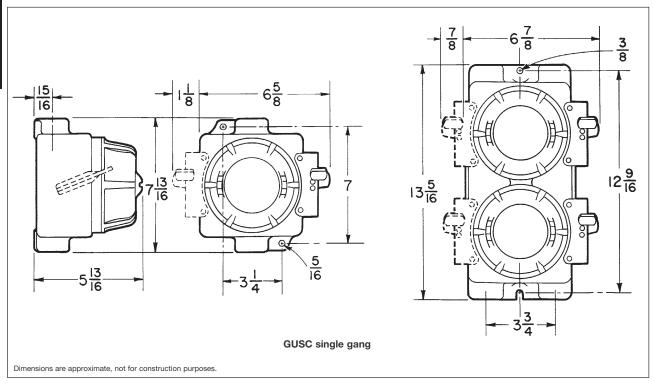
$\uparrow$ See listings for catalog numbers which are suitable for use in Group B hazardous locations. Seals must be installed within  $1\frac{1}{2}$ " of all conduit openings. Quicklag is a registered trademark of Cutler-Hammer Inc.
