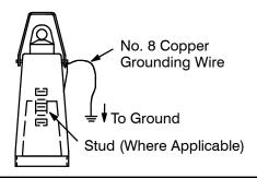
In new installations, where the bushing is known to be de-energized, thoroughly wipe the bushing interface and the insulated cap interface clean of all contaminants. Lubricate above surfaces with the supplied lubricant or Elastimold approved lubricant. On circuits previously energized, clean and lubricate only the interface of the insulated cap.
