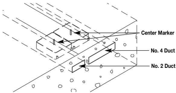
**Step 2.** Mark concrete with cutting lines based on single-, double-, or triple-gang afterset to be installed. Opening should be approximately 1/2" [12.7mm] wider than the afterset on all sides. Drill a 2 1/2" [64mm] diameter hole over the center of the duct to determine depth of concrete if depth is not known. Set saw to depth of concrete and cut opening for the afterset.
