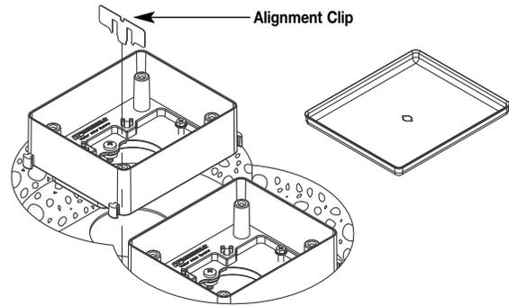
**Step 7.** Install mudcaps and fill space around afterset and mudcaps with grout. using trowel, create level, smooth surface.
