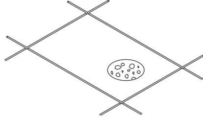
**Step 3.** Loosen and remove concrete slugs.
