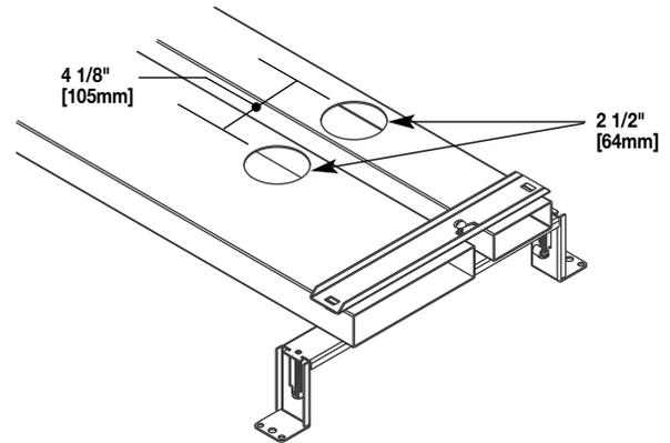
**Step 3.** Place the presets directly over the holes. Connect the presets together with the alignment clips. Secure the preset to the duct by tightening the locking tabs.
