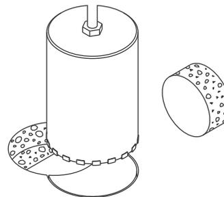
**Step 5.** Using a 2 1/2" [64mm] diameter hole saw, drill opening in center of duct. For two- or three-gang, use template for proper center locations.
