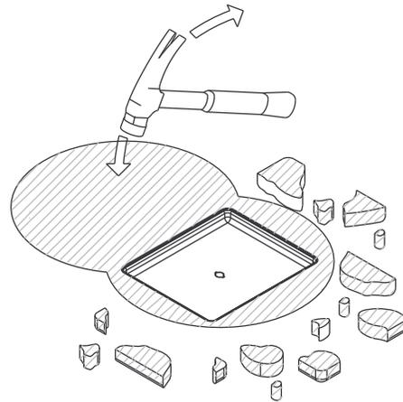
**Step 9.** Remove mudcaps and replace carpet. Using the afterset as a guide, cut a rectangular opening in the carpet. Attach desired service fitting.
