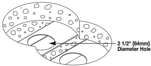
**Step 6.** Attach afterset to the duct system by tightening locking tabs. Secure aftersets together with alignment clip (two- or three-gang only).
