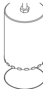
**Step 3.** Loosen and remove concrete slug.
