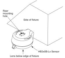
The sensor should be positioned below the fixture edge and away from fluorescent lamps so that lamp heat does not affect the sensor.
