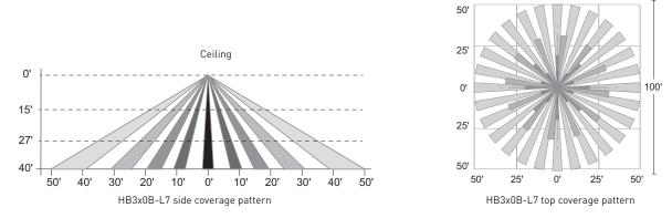
For high bay applications, the HBL7 is designed for mounting at heights between 20' to 40', with a coverage area up to 100' in diameter when mounted at 40'.
