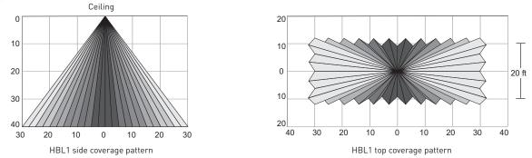
The HBL1 is designed to detect walking motion when mounted at 40' above the floor. When mounted at 40', in optimal conditions, the lens has a 60' linear detection range.
