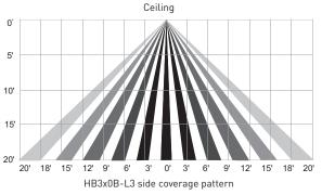
For mid bay applications, the HBL3 pattern spreads over a 40' diameter area at a height of 20'.
