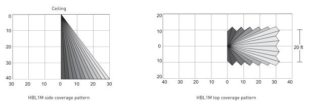
Identical to the HBL1, the HBL1M comes with opaque adhesive tape applied to the interior of the lens, cutting off 1/2 of the coverage pattern. This customized coverage is ideal for the beginning of aisle ways where cross traffic could be an issue.
