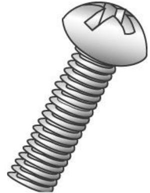
*A straight shank fastener with external threads designed to go through a hole or nut that is pre-tapped to form a mating thread for the screw.*
