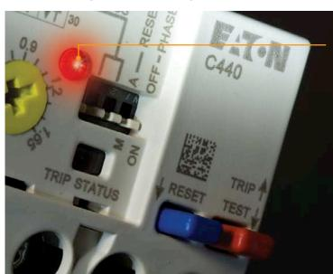
Single blink: Normal operation Double blink: Fault condition developing
