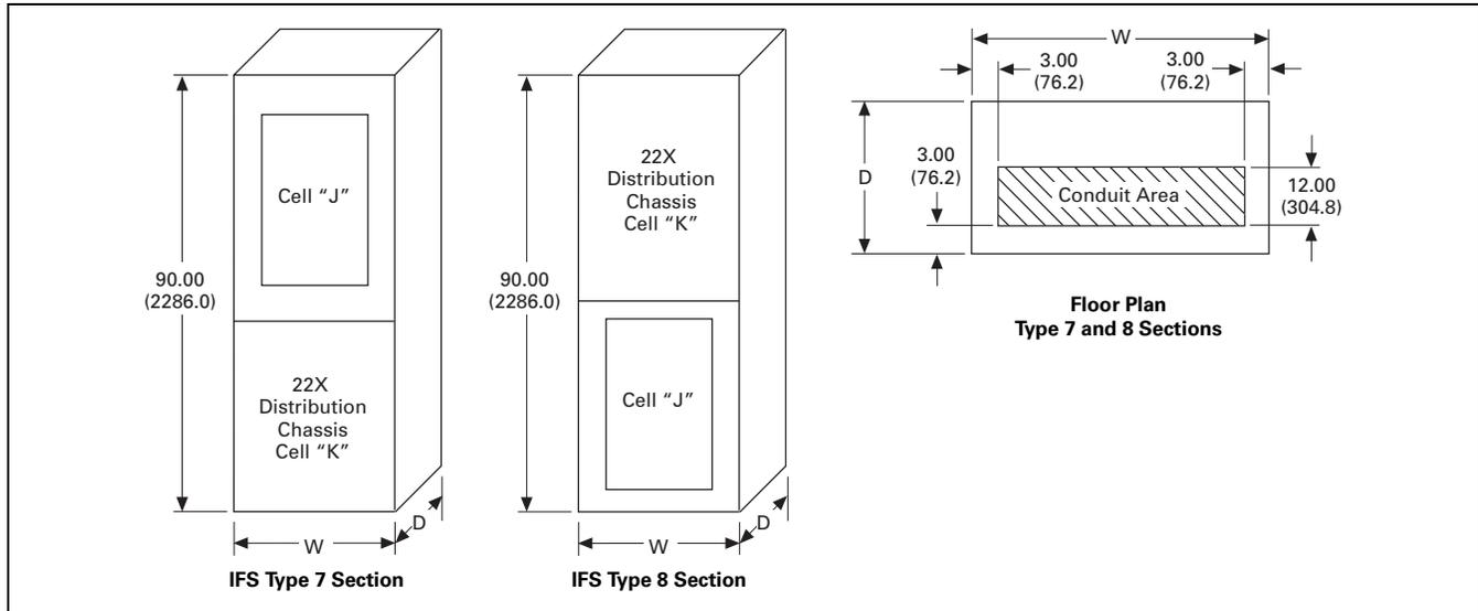
Figure 21.6-7. Type 7 and 8 Integrated Facility System Switchboards Distribution Section Layout—Dimensions in Inches (mm)
