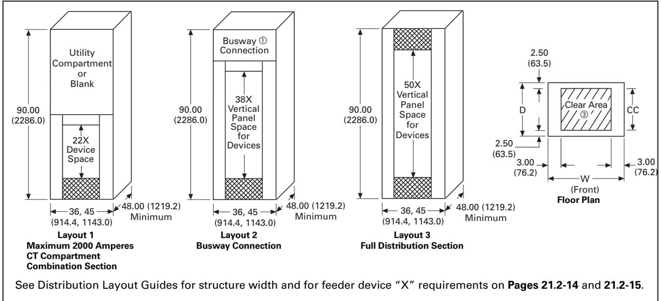
**Figure 21.2-10. Distribution Section Layout—Dimensions in Inches (mm)**
