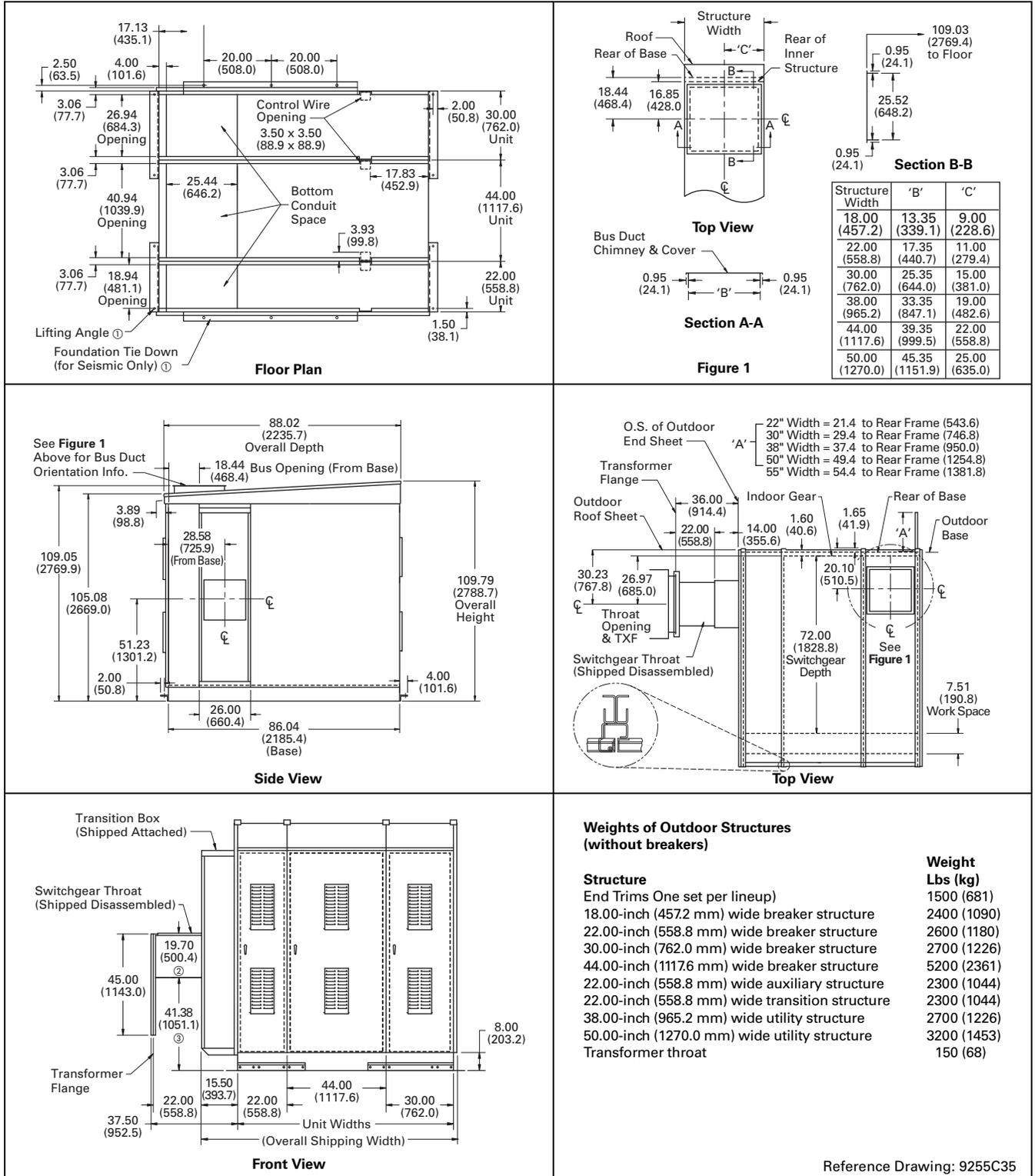
**Figure 21.5-13. Outdoor Non-Walk-in Enclosure Dimensions in Inches (mm)**
