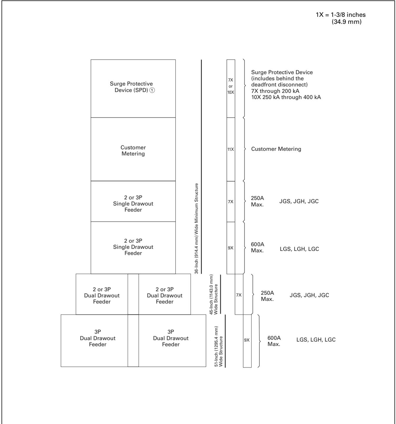
**Figure 21.1-10. Circuit Breaker “X” Space Requirements—Dimensions in Inches (mm)**
