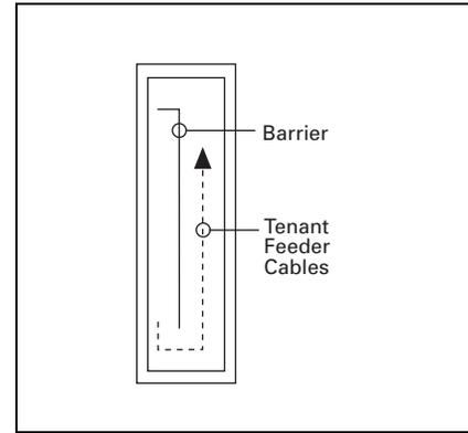
**Figure 21.10-8. Rear Barriered Wireway Metering Section Side View**
