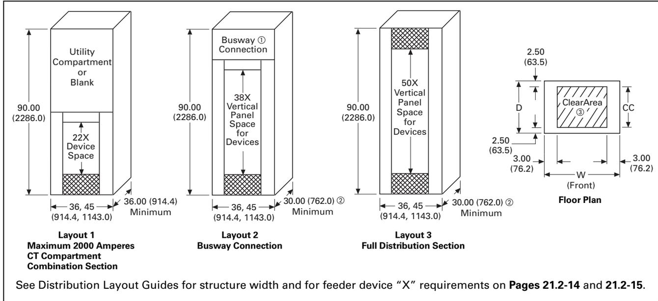
**Figure 21.2-9. Distribution Section Layout—Dimensions in Inches (mm)**
