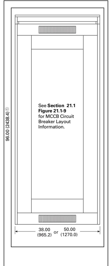
**Figure 21.5-9. Group-Mounted Molded Case Circuit Breaker Switchboard**
