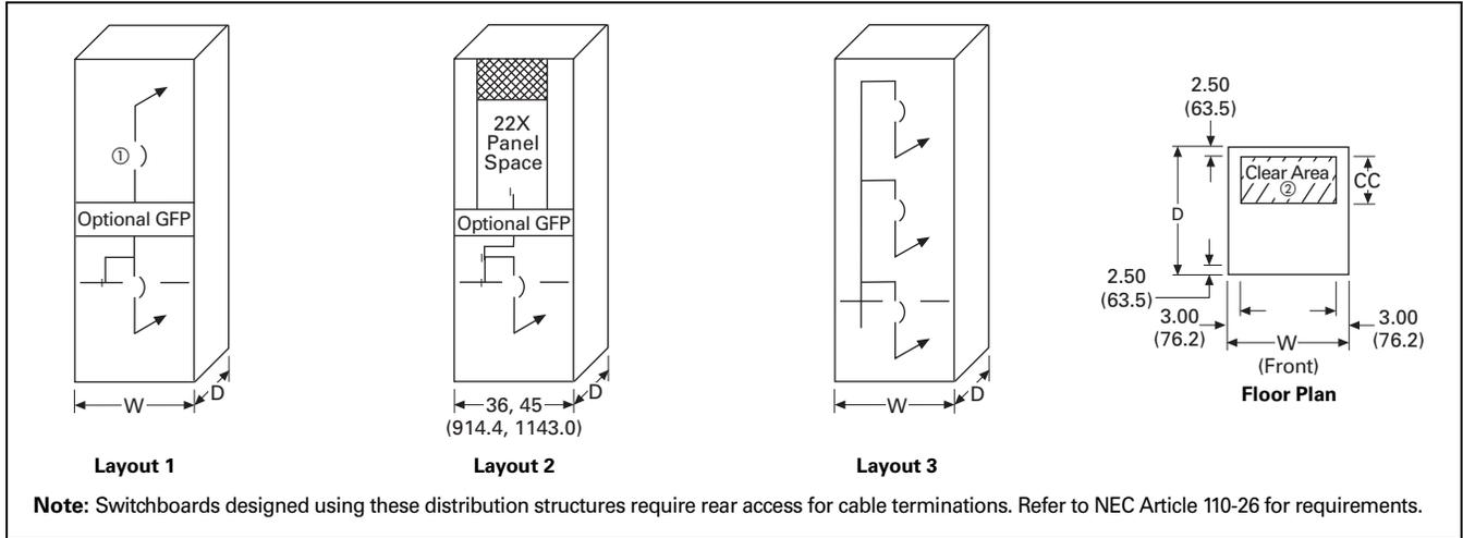
Figure 21.2-8. Individually Mounted Feeder Layouts—Dimensions in Inches (mm)
