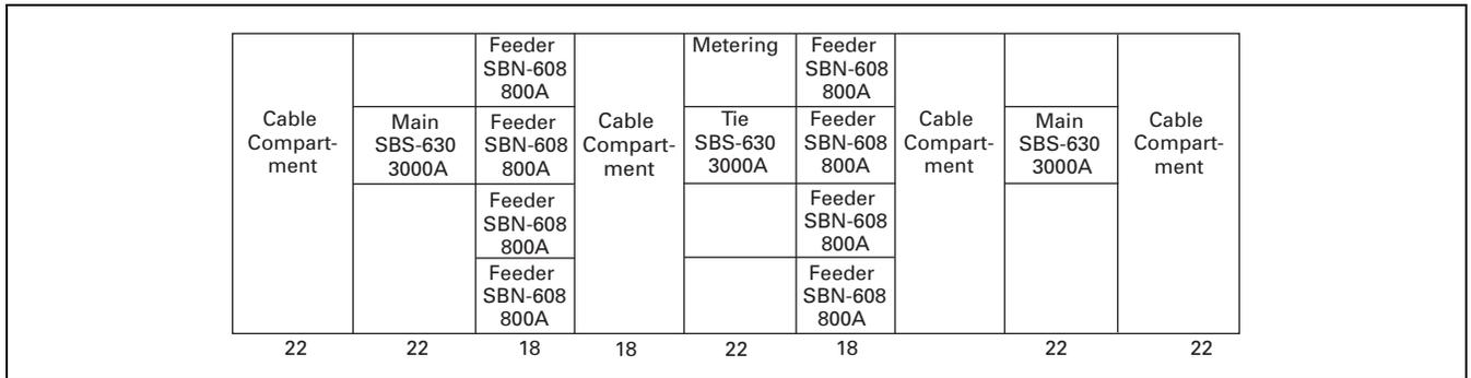
**Figure 21.5-5. Standard and Narrow Breakers—Typical Main-Tie-Main Layout**
