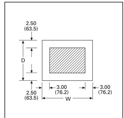
**Figure 21.10-13. Typical Conduit Area—Figures 21.10-10, 21.10-11 and 21.10-12**
