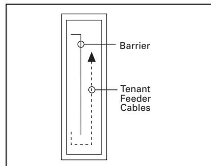
**Figure 21.10-18. Rear Barried Wireway Metering Section Side View**
