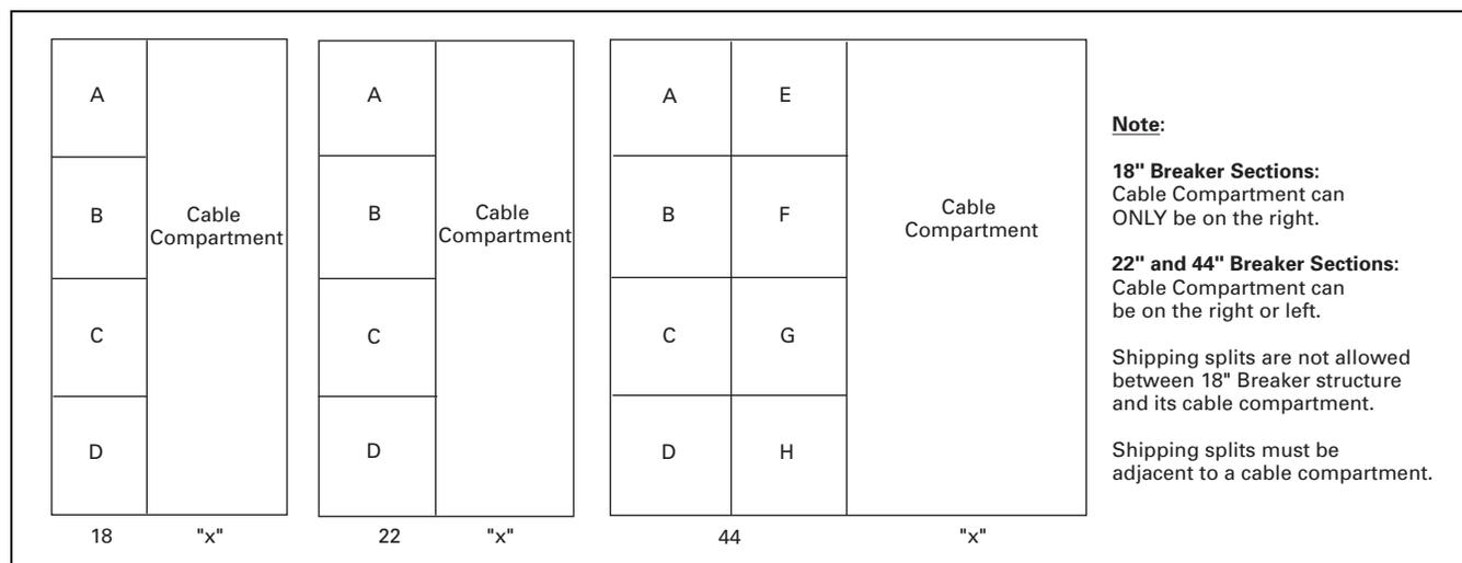
Figure 21.5-3. Breaker Structures
