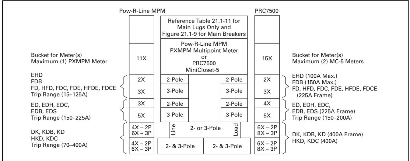
Figure 21.9-3. PRL MPM / PRC7500 Layout Guide for Current Sensor and Current Transformer Sizing—Standard Pow-R-Line C Switchboard Construction Applies
