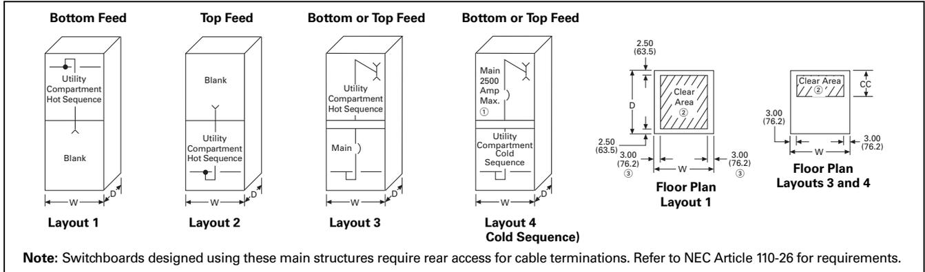
**Figure 21.2-1. Utility Compartment Layouts—Dimensions in Inches (mm)**
