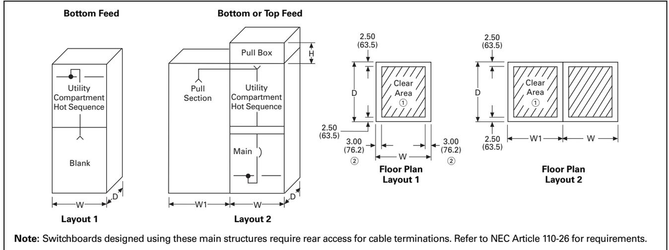
**Figure 21.2-3. West Coast Utility Layouts—Dimensions in Inches (mm)**
