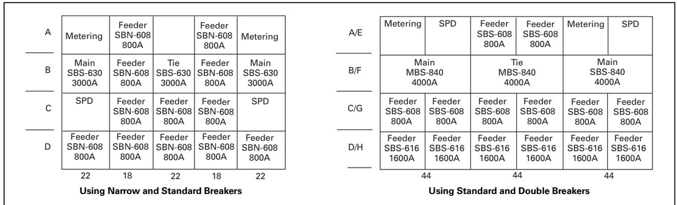
**Figure 21.5-2. Main-Tie-Main Typical Layouts**
