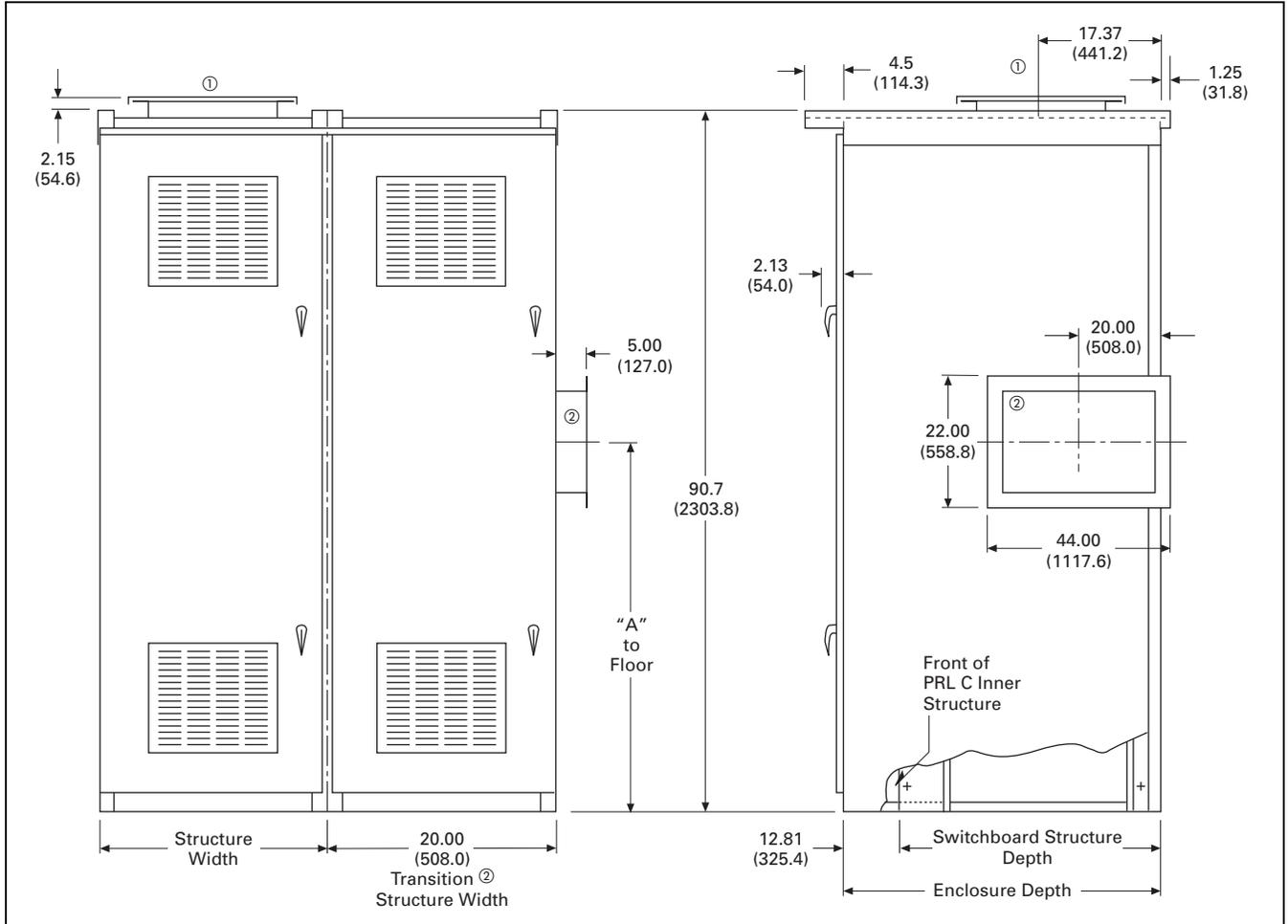
**Figure 21.4-1. Front-Access—Non-Walk-In with Flat Roof—Dimensions in Inches (mm)**
