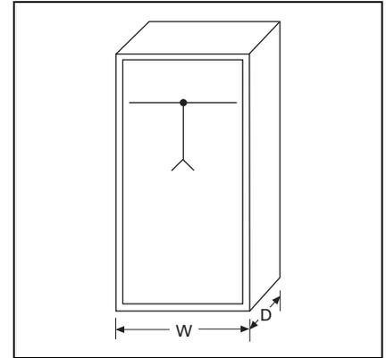
**Figure 21.10-2. Main Lugs Only—Top or Bottom Feed**
