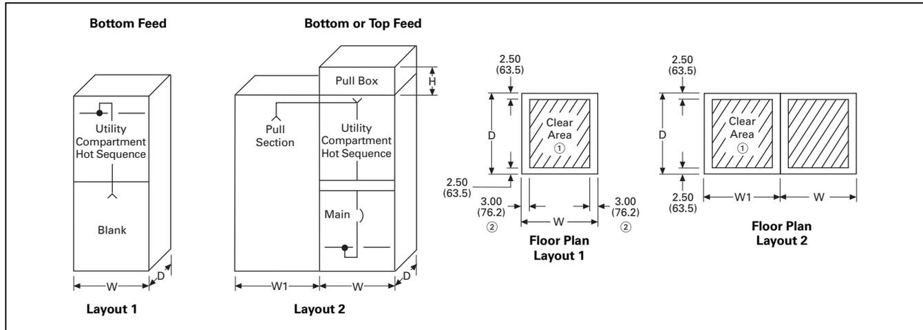
Figure 21.1-3. West Coast Utility Compartment Layouts—Dimensions in Inches (mm)
