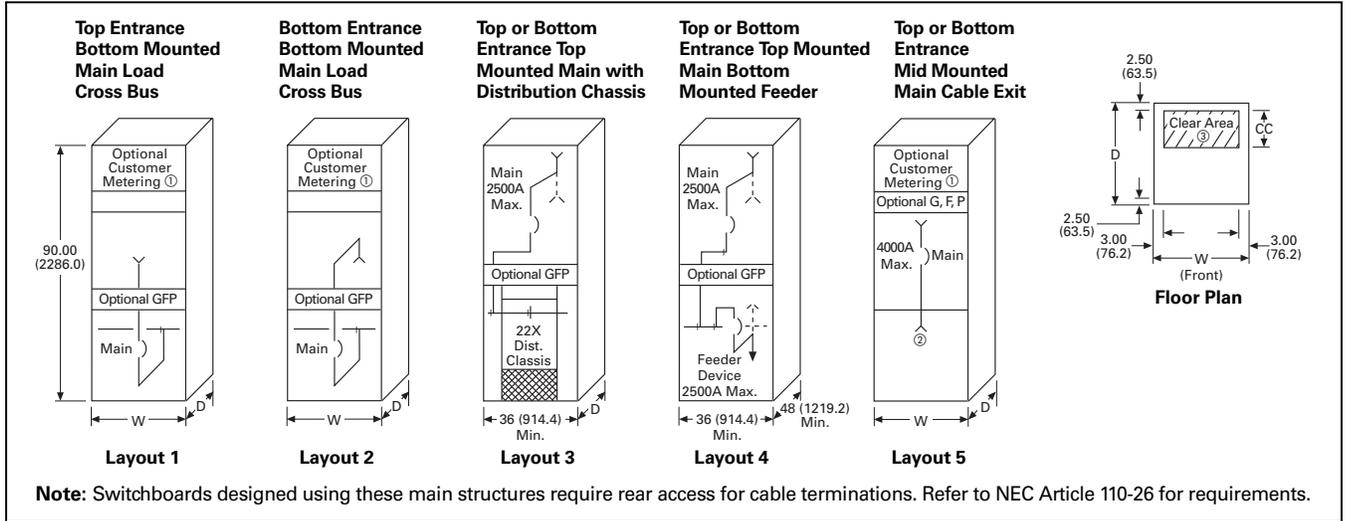
**Figure 21.2-6. Main Section Layouts—Dimensions in Inches (mm)**
