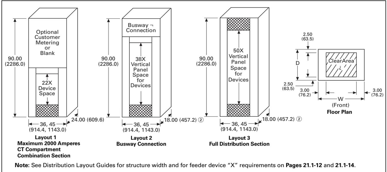
**Figure 21.1-7. Distribution Section Layouts—Dimensions in Inches (mm)**
