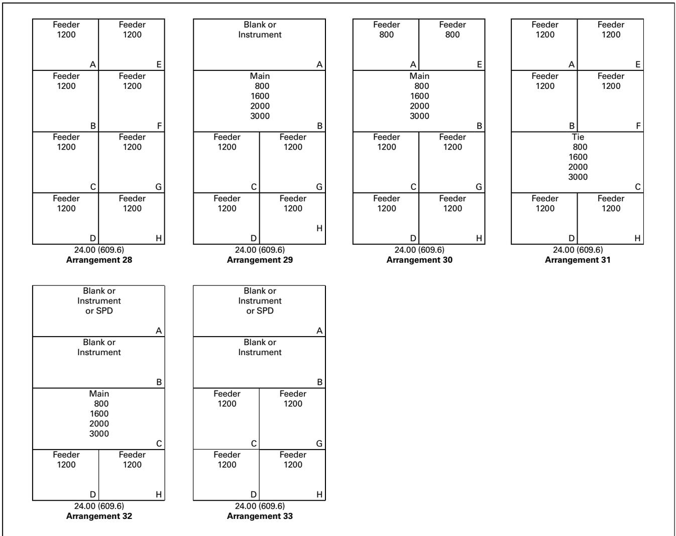
**Figure 21.6. Typical Structure and Breaker Arrangements (Continued)—Magnum SB Mains and Ties, and Series NRX Feeder Breakers—Dimensions in Inches (mm)**
