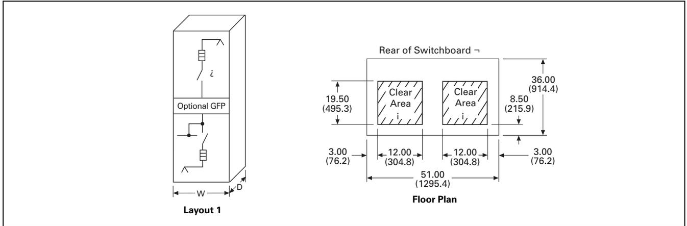
**Figure 21.1-12. Individually Mounted Feeder Layout—Dimensions in Inches (mm)**
