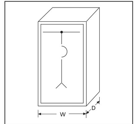
**Figure 21.10-3. Main Device (Breaker or Switch)—Bottom Feed**
