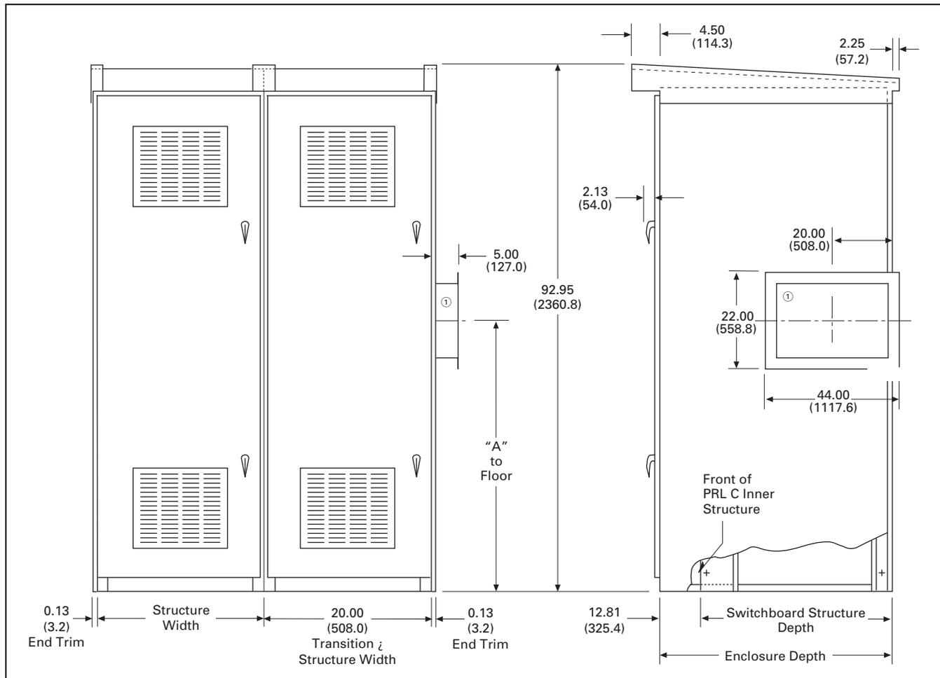
Figure 21.4-2. Front-Access—Non-Walk-In with Sloped Roof—Dimensions in Inches (mm)
