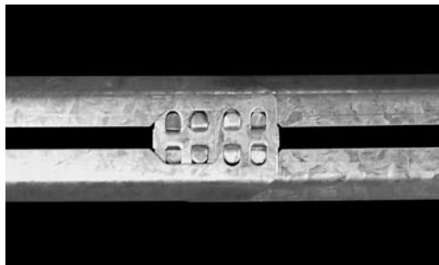
(After inserting into brackets {A} on housing) Assemble the bar hangers by overlapping the ends of the two sections and placing the tabs on each section into the square hole in the opposite section.
