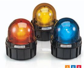
Federal Signal Model 371 incandescent warning lights have a powerful sealed beam lamp that rotates 360° within a glass dome. The lamp itself is mounted in a pivoting yoke. This allows the lamp beam angle to be adjusted through 90° from horizontal to vertical. Changing the beam angle allows the user to create unique light patterns and/or direct the light for better visibility.
