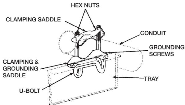
1. Remove any non conductive coating from surface of conduit at clamp contact points prior to installation.
