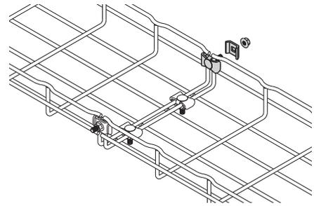
1 Install one kit on each side and remaining kit(s) on bottom.
