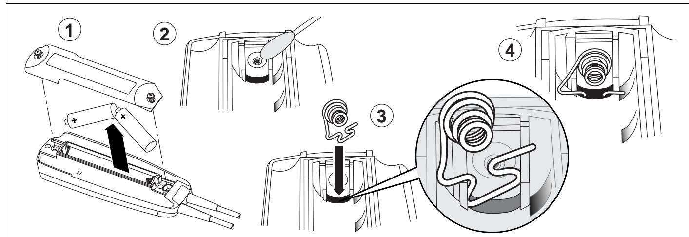
**Purpose:** Retrofit of T2 battery contact.
