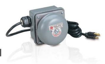
Federal Signal's TELB TelCom® Extension Ringer Bell is a vibrating bell activated by the ringing signal of a telephone system. The TELB is specifically designed for use with an analog telephone. The ringing signal of 40-150VAC, 16-60Hz and local 120VAC power is all that is required to activate a TelCom signal.
