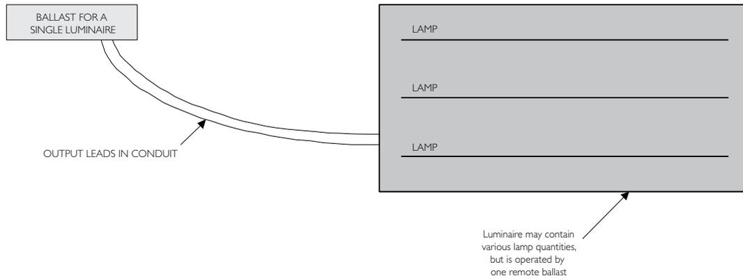
Note: Recommended output lead lengths and remote mounting distances should not be exceeded.
