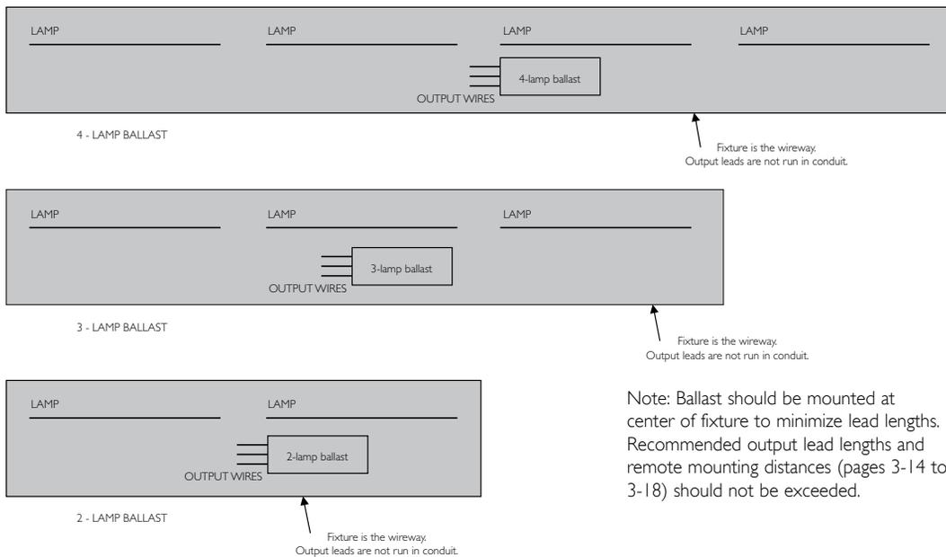
Note: Ballast should be mounted at center of fixture to minimize lead lengths. Recommended output lead lengths and remote mounting distances (pages 3-14 to 3-18) should not be exceeded.
