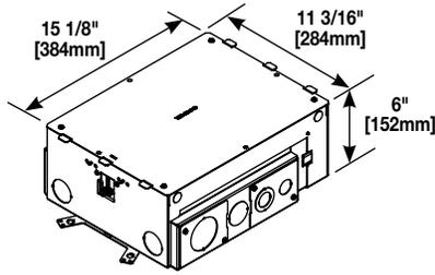
**10-Gang Floor Box** – has been designed to be installed in concrete floors, raised floors, & wood floor applications. Box has a fully finished interior to assist plugging and unplugging of devices. **Box comes complete with all components needed for initial installation.** Box is compatible with Wiremold® Walkerflex Modular Wiring System. Custom options are available upon request.
