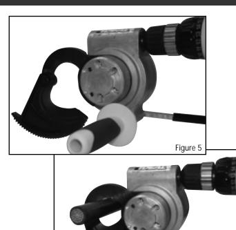
STEP 5: Place the cable to be cut onto the stationary blade and close the moving blade around the cable. Feed the moving blade by hand until the first gear teeth are engaged (Figure 5 and 6).
