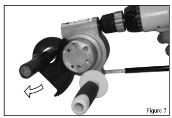
**STEP 7:** To cut several small cables continuously, cut first cable as described above, then reverse blade until opening is sufficient to feed the next cable through. Continue to alternate between forward and reverse modes until all cables are cut (Figure 7).
