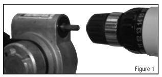
**STEP 1:** Attach cable cutter drive shaft to drill as shown (Figure 1). Tighten drill chuck securely.
