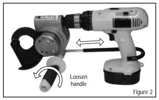
STEP 2: Loosen handle so torque arm extends freely (Figure 2).
