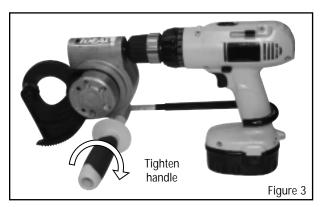
STEP 3: Loop torque arm around drill handle and tighten handle into locking collar to lock torque arm in place (Figure 3). Do not operate tool without torque arm in place.
