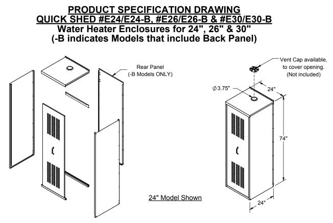
The HOLDRITE® QUICK SHED<sup>™</sup> Water Heater Enclosures are constructed of galvanized steel and provide protection for water heaters installed in outdoor locations. Anchor points at the rear of the enclosure allows for optional attachment to the adjacent building structure. Rear panel (-B version ONLY) provides a four-sided enclosure.
