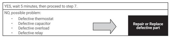
7. Make sure the coils are clean. Then check evaporator "air in" and "air out" temperatures. If the temperatures are the same:
