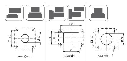
Caution: The mounting surface must be smooth and flat. If not avoided, it is possible that problems of load, adjustment and protection class arise.
