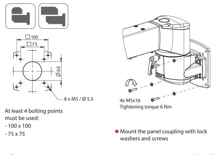
When using panel coupling components, always ensure that the stability of the mounting surface is suitable for mounting. Attention
