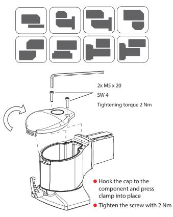
Indication: Mounting and dismounting of the component "elbow" is illustrated below
