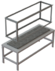
Lower frame over mounting subpanel
