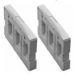
Suitable for the 1140-mm² Triple-T profile. Use to fasten the busbars to a backpanel or modular enclosure system structure. The supports also serve as bracing against the forces present during short circuit conditions.
