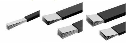
Flat, flexible busbar complements the space-saving nature of the 60-mm busbar system. Unlike traditional round conductors, flexible busbar can be folded and shaped without regard to AWG bending radius issues. Choose connection sets that are designed to accept flexible busbar, or drill the flex for use with a stud connection (on your breaker, VFD, SCR or other system component.)
