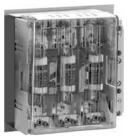
Blade size Class J bus-mounting fuse holders in 100 A, 200 A and 400 A frame sizes. Connection on bottom or top, 3-pole, 30 x 10, Double-T and Triple-T busbar sections.
