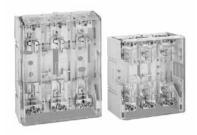
UL Class J 100 A, 200 A and 400 A panel-mount fuse holders. Clear plastic cover satisfies IP20 touchsafe design standards. The only 3-pole blade size Class J fuse holder in the industry with integral touchsafe cover.
