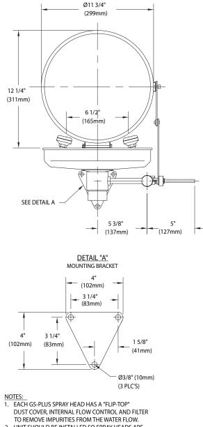
2. UNIT SHOULD BE INSTALLED SO SPRAY HEADS ARE 33"-45"(838mm-1143mm) ABOVE FINISHED FLOOR.
