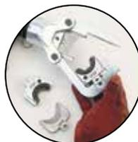
**2** Alternate die adapters, cutter blades, or knockout punch adapters slide right in!
