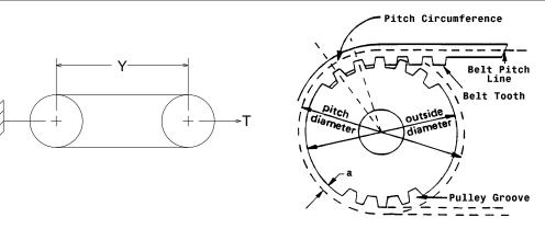
The length shall be measured by placing the belts on two pulleys of equal diameters that have been grooved in accordance with standard specifications and rotated at least three complete turns with the specified tension so that each strand receives half the total tension. The length will be that length obtained by adding the Pitch Circumference of one pulley to twice the center distance (dimension 'Y').
