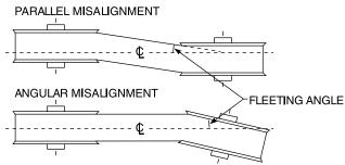
There are three possible causes and solutions of sheave or sprocket misalignment:
