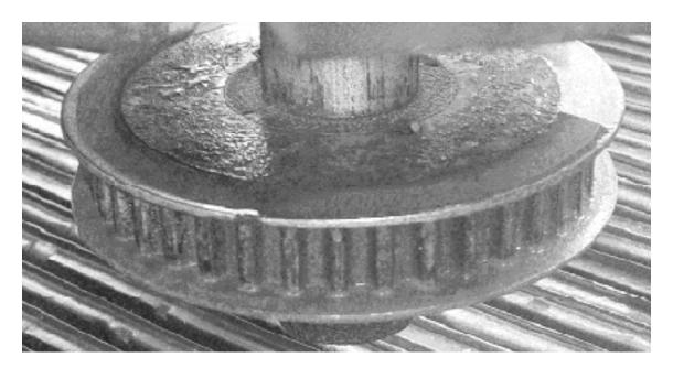
Sprockets with corrosion in the grooves will rapidly wear the belt's teeth. Sprockets with corroded grooves will wear through the abrasion resistant tooth fabric, resulting in tooth shear and premature belt failure.
