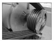
Using EZ Align® laser alignment tool showing laser line on target
