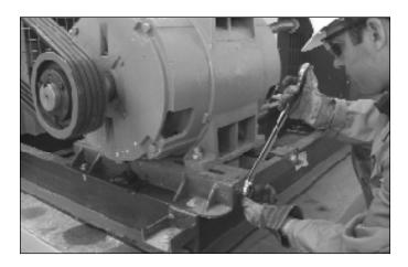
4. Move the motor in until the belt is slack and can be removed easily without prying. Never pry off a belt, as the sheave or sprocket can be damaged. Prying off belts also adds the risk of injury.
