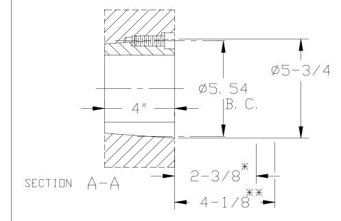
\* SPACE REQD TO TIGHTEN BUSHING ALSO SPACE REQD TO LOOSEN SCREWS TO PERMIT REMOVAL OF HUB BY PULLER.
