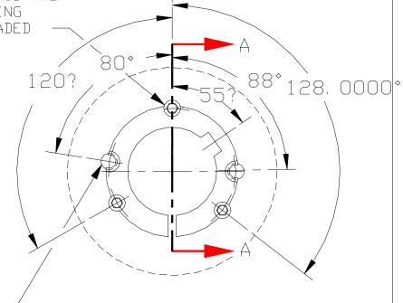
·USE ONLY TWO SCREW FOR REMOVING FROM SHAFT: BUSHING HALF OF HOLE IS THREADED-HUB HALF OF HOLE IS NOT THREADED BNRF: BUSHING KW:
