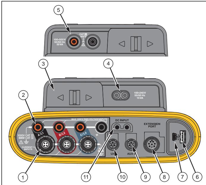
**Figure 7. Connector Panel**
