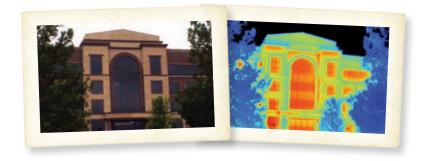
Energy losses are common in commercial buildings and industrial facilities. While there can be a number of culprits, such as air leaks or systems running inefficiently, many energy losses can be detected through inspection with thermal imaging.
