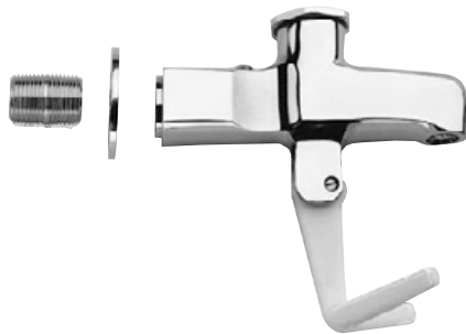
#10200 – Glass Filler Head: 3/8”F w/ 3/8” close nipple, flange, locking compound (Replacement head for Fisher and T&S Glass Fillers – replaces Fisher #1000, #1001, and #1005)
