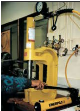
◀ A-310 Arbor Press used for compacting powder at 10 ton.
