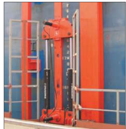
▼ Each climbing unit consists of two 70 tons double-acting cylinders and two 20 tons locking cylinders.
